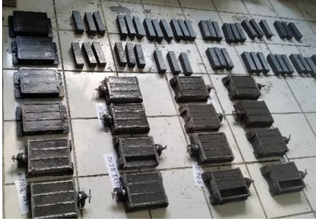
Figure 1. Preparation of concrete specimens
