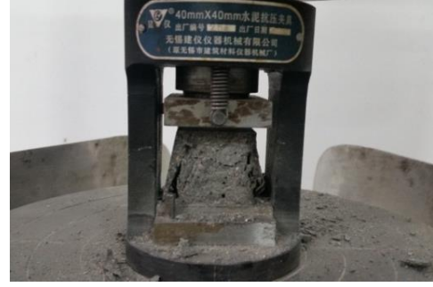
Figure 2. Compressive strength testing
