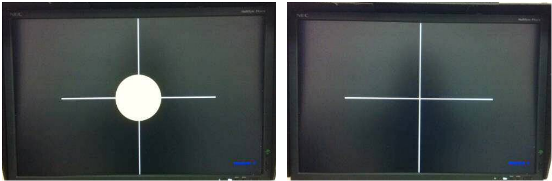
Figure 3.7. A representation of the participant's view of the circular stimulus (left panel) and the fixation target alone (right panel) as seen on the NEC MultiSync PA24/W VDU monitor.
