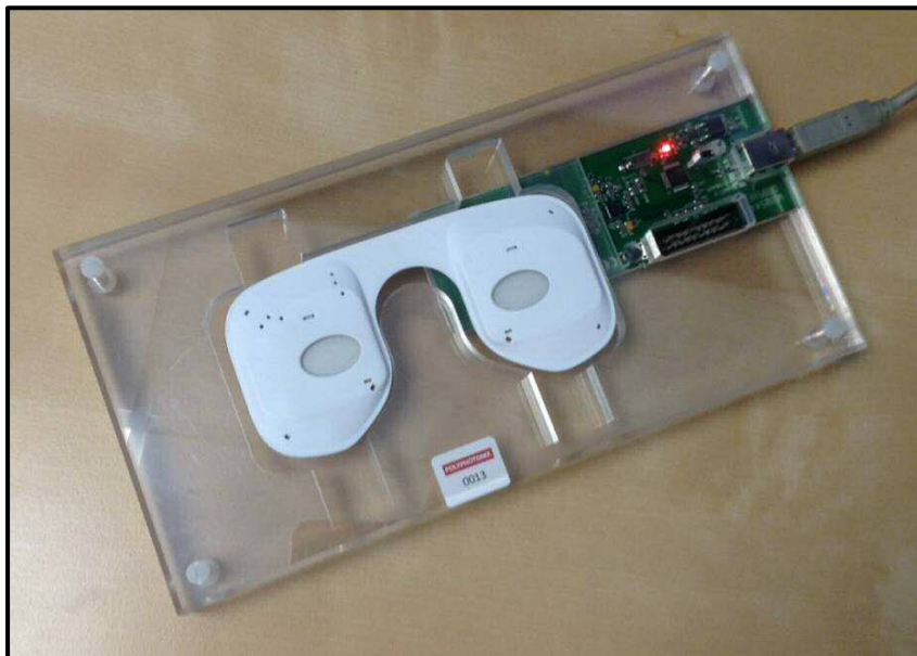
Figure 3.3. A photograph of the hardware used to connect each mask to the PPX Works program. This system was used to program a mask before use, download compliance data at each monthly follow-up visit and record the return of a mask after 3 months wear.
