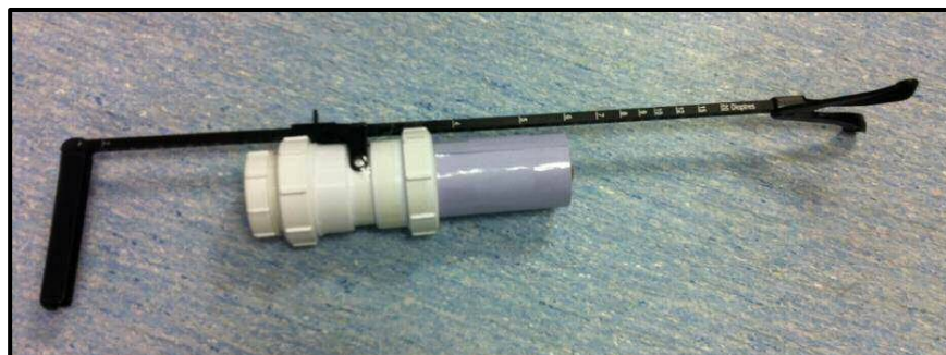
Figure 3.9. A photograph of the bleaching source setup. The portable device was mounted onto a modified RAF rule and connected to a mains voltage supply for use.
