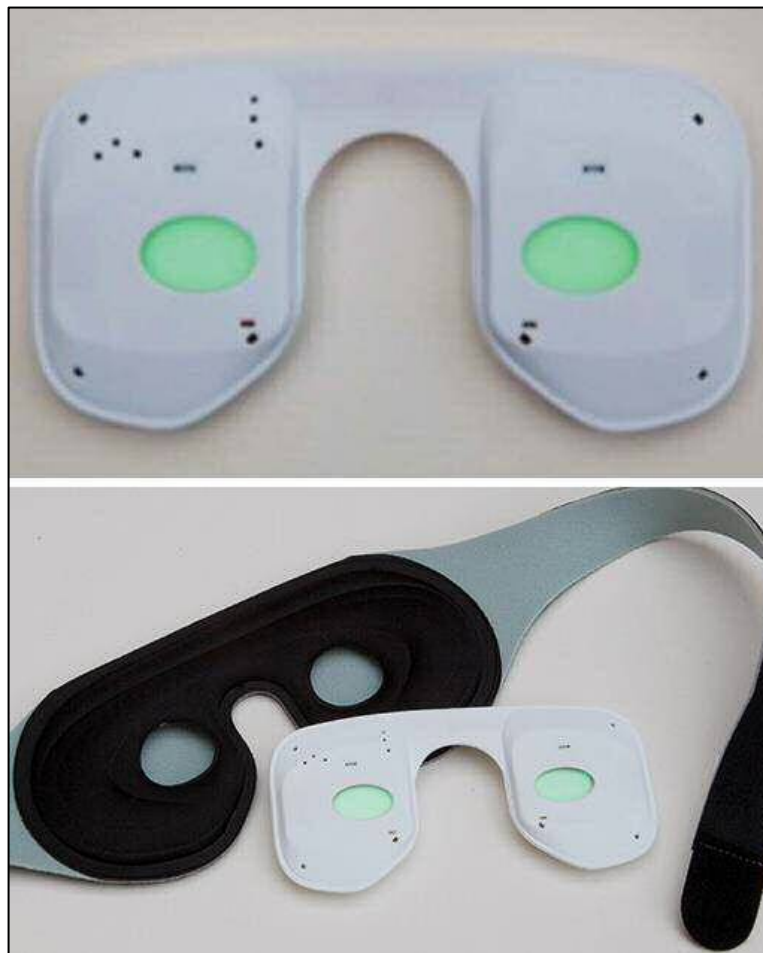
Figure 3.2. Principle components of the OLED sleep mask. The top panel shows the light-emitting 'pod' of peak output 502 nm. The bottom panel shows the cushioned fabric mask that houses the pod.
