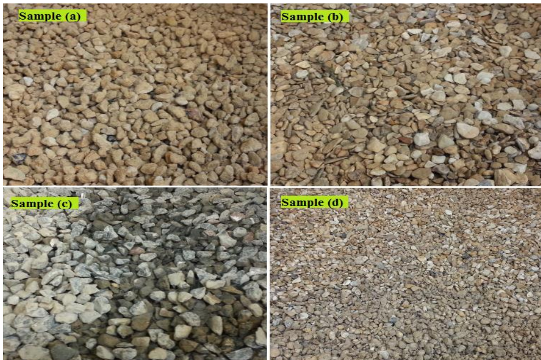
Figure 7.1: Photographs of the four types of gravel: (a) 20 mm Cotswold buff decorative stone chippings. (b) 20 mm limestone chippings. (c) 20 mm bulk gravel. (d) 10 mm bulk gravel.
