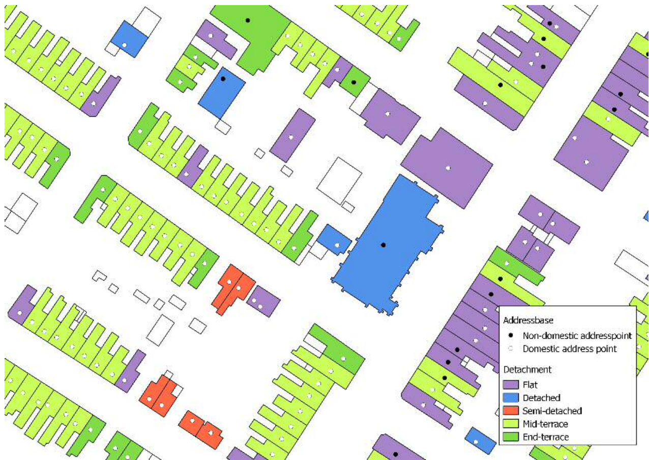
Figure 18: Applying building data to UPRNs in GIS
