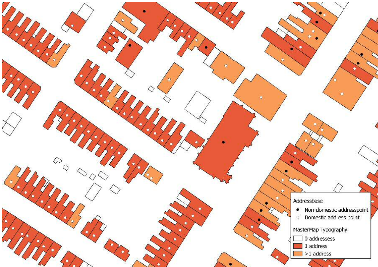
Figure 14: GIS database formation (addressbase premium and mastermap topography layer)
