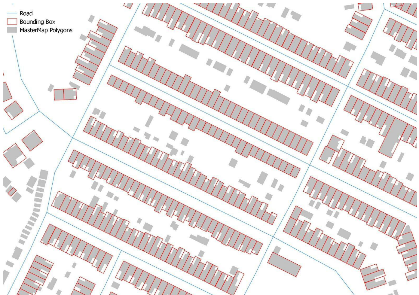
Figure 17: Determining buildings' perimeter ratio using GIS
