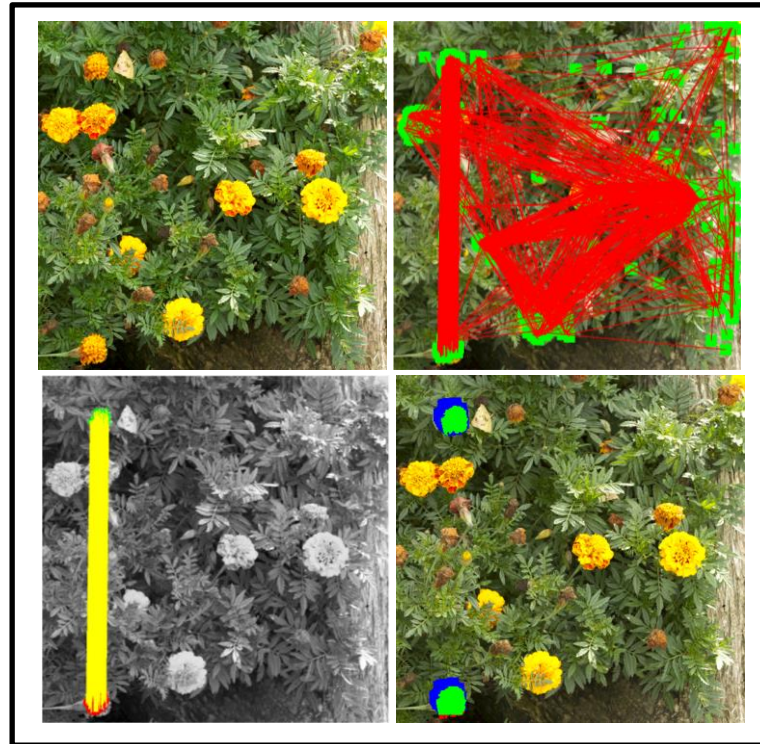
Figure 3-26: An example of detecting duplicated scaled objects using improved DSIFT: (top to bottom, left to right) Forged image, copied object scaled up by 10%, primary detection, RANSAC result, final result after hysteresis.
