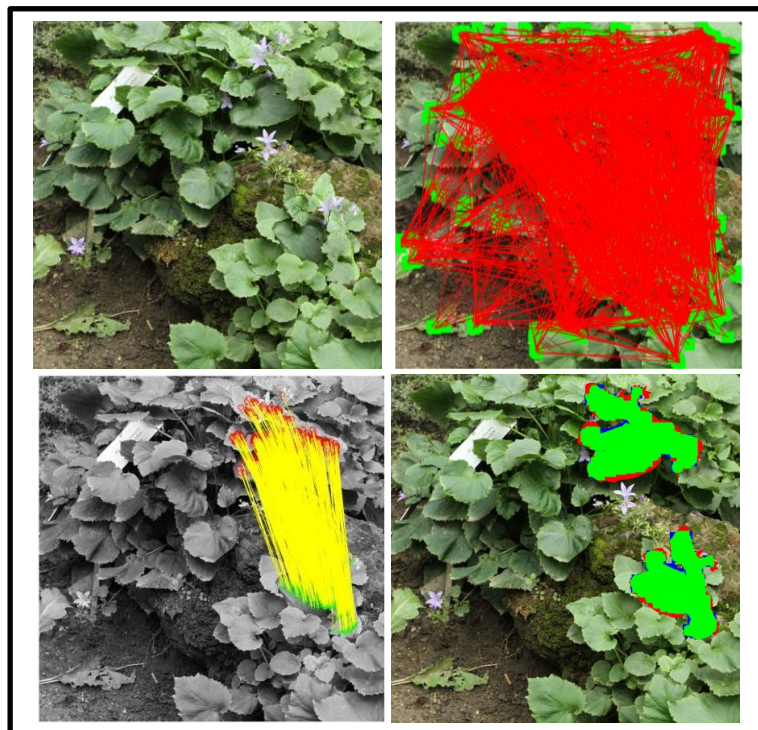
Figure 3-32: An example of detecting duplicated scaled objects using improved DSIFT: (top to bottom, left to right) Forged image, copied object scaled down by 15% and rotated by 45°, primary detection, RANSAC, final result after hysteresis.
