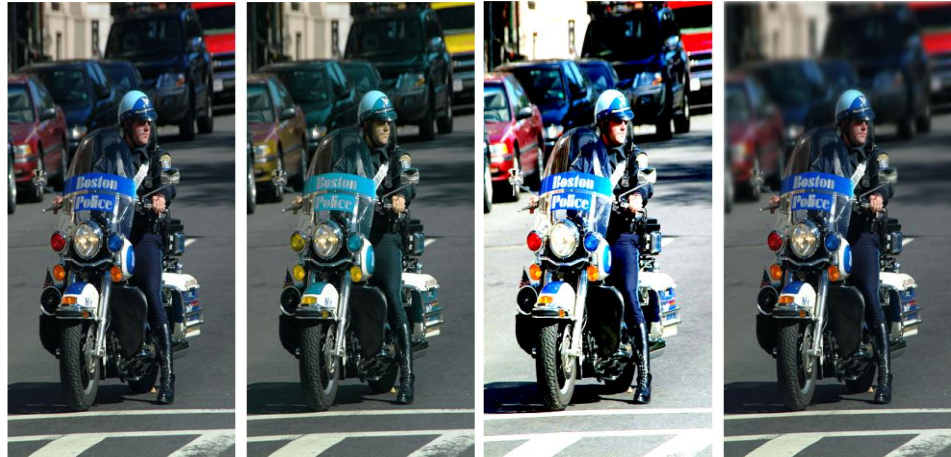
Figure 2-8: (left to right) an original image, the image enhanced to alter the colour, contrast, and blur of the background cars[14].
