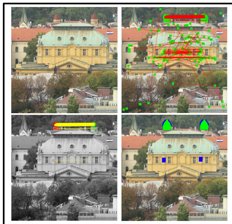
Figure 4-22: An example of detecting duplicated scaled objects using FFRID: (top to bottom, left to right) input forged image, copied object scaled up by 5% and vertically skewed by 1%, primary detection, RANSAC result, final result after hysteresis.
