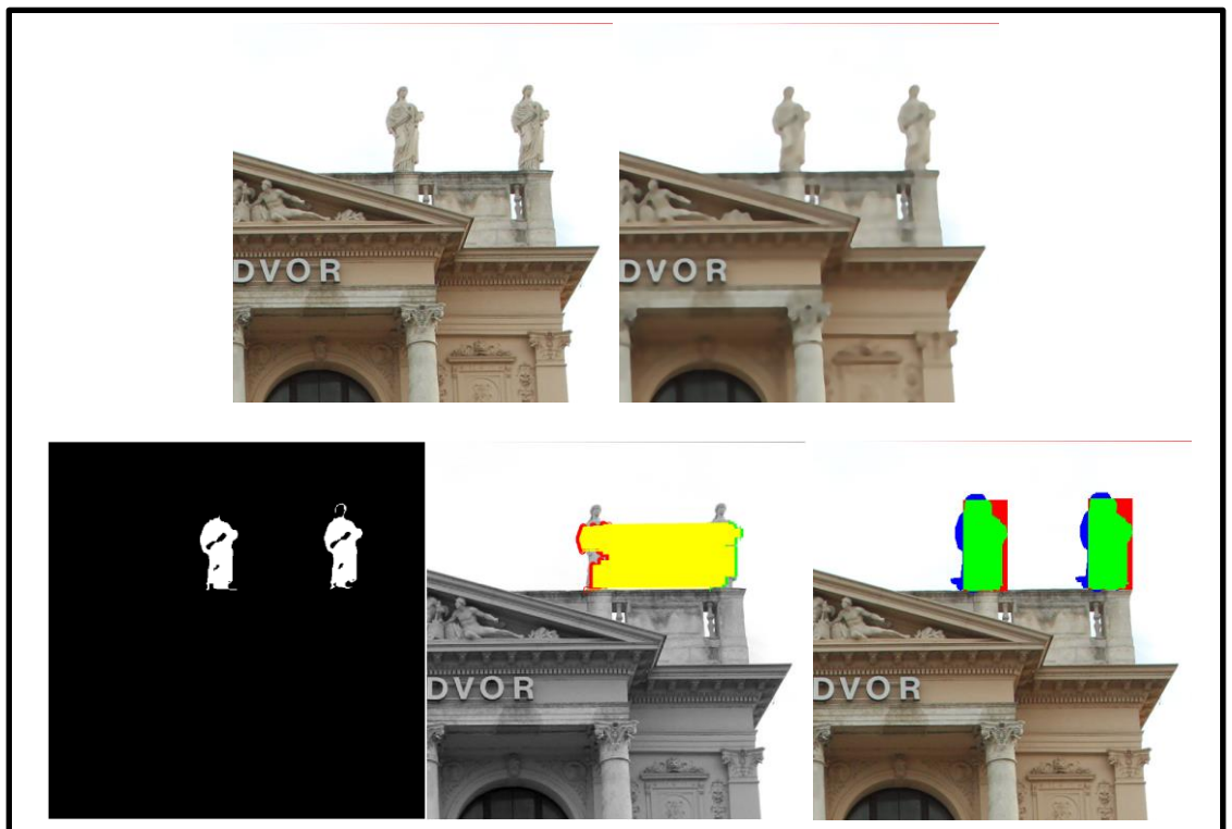
Figure 5-17: (top to bottom, left to right) input forged image, Rolling Guidance image, primary detection, RANSAC result and final result after hysteresis.
