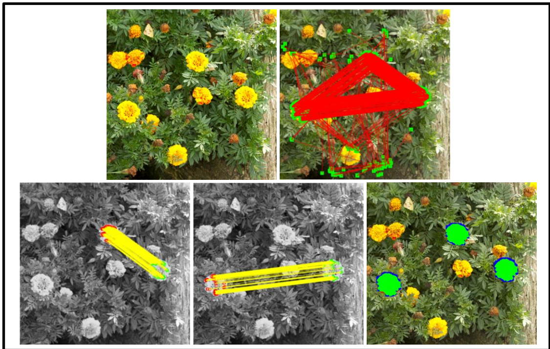
Figure 4-23: An example of detecting multiple duplicated objects using FFRID: (top to bottom, left to right) input forged image, copied objects (horizontally elongated by 3% and vertically skewed by 2%, vertically elongated by -5% and horizontally skewed by 3%), primary detection, RANSAC result, RANSAC result, final result after hysteresis.
