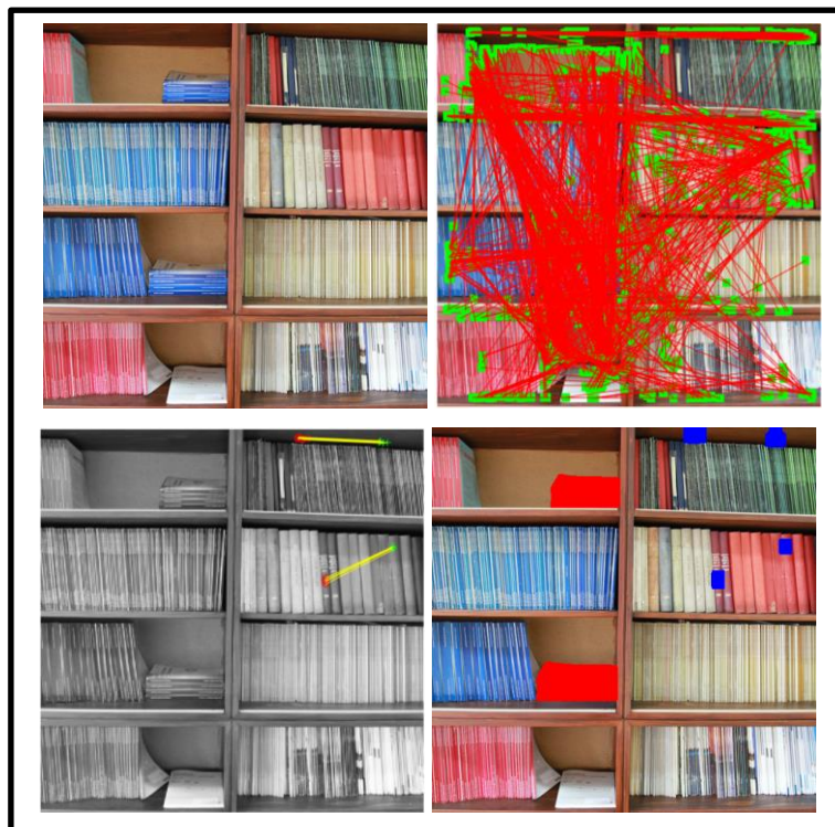
Figure 4-16 An example of failure of detecting duplicated scaled objects using FFRID: (top to bottom, left to right) input forged image, copied object scaled down by 15%, primary detection, RANSAC result, final result after hysteresis.
