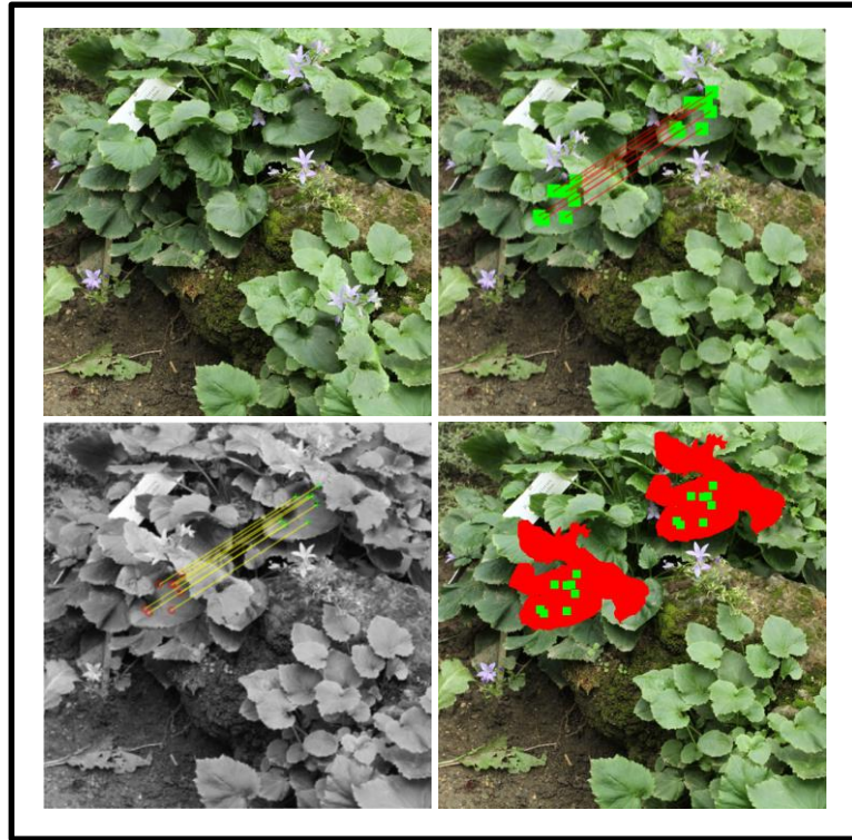
Figure 3-40: detecting multiple duplicated objects using improved SIFT on flat region (top to bottom, left to right), SIFT keypoints with refinement step, SIFT keypoints with refinement step, primary detection, Final result.
