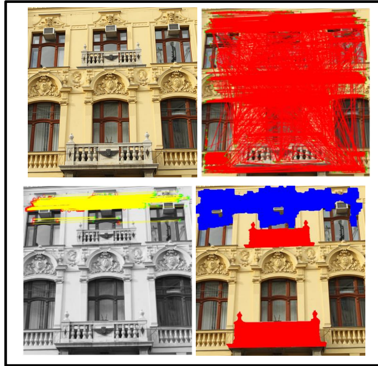
Figure 3-35 An example of failure of detecting duplicated scaled objects using improved DSIFT: (top to bottom, left to right) Forged image, copied object scaled up by 70% and rotated by -1%, primary detection, RANSAC result, final result after hysteresis.
