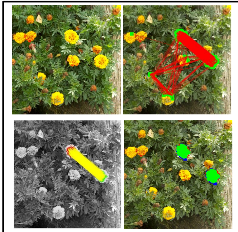
Figure 3-28: An example of detecting duplicated scaled objects using improved DSIFT: (top to bottom, left to right) Forged image, copied object with a vertical skew factor of 8%, primary detection, RANSAC result, final result after hysteresis.
