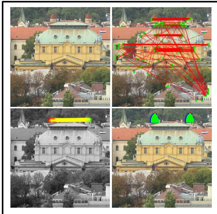
Figure 3-33: An example of detecting duplicated scaled objects using improved DSIFT: (top to bottom, left to right) Forged image, copied object scaled up by 5% and vertically skewed by 1%, primary detection, RANSAC result, final result after hysteresis.
