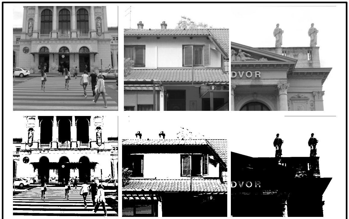
Figure 5-9: an example of using Otsu's method to convert a grayscale image to a binary image.
