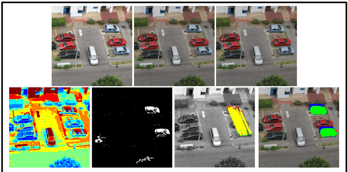
Figure 5-29: (top to bottom, left to right) Input forged image with copied object rotated by 5^\circ , Forged image after Contrast Adjustment, Rolling Guidance image, Quantized image, Primary detection, RANSAC result and final result after hysteresis.
