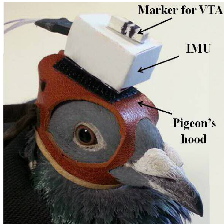
Figure 6-7 IMU placement on the pigeon's head. a custom made leather hood is used to velcro-mount the IMU to the pigeons head without obscuring its field of view.
