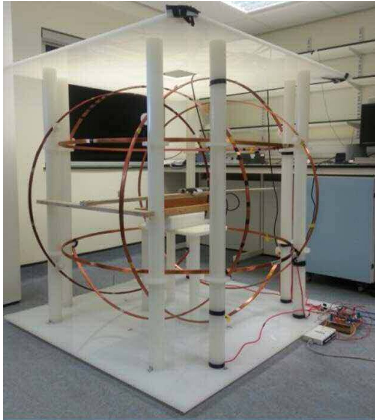
Figure 2-19 A picture of the constructed 3-D Helmholtz coil system
