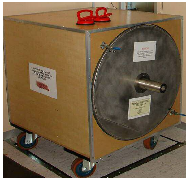
Figure 2-10 Chamber passive shielding.
