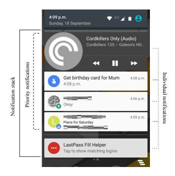
Figure 7.1: A typical Android notification drawer showing an example stack of notifications. Priority notifications refer to those with a priority (set by the application) of at least "Normal" [3], discussed further in Section 7.2.
