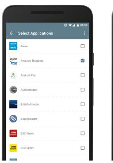
(a) The application rule interface that allows users to select which applications to receive save prompts for after notifications are removed. This screen is shown in the setup and accessed from the main menu thereafter). (b) Boomerang Notifications' settings interface that is accessible from the main menu. Settings include allowing users to activate/deactivate the application and set additional preferences regarding saving notifications and reminders (outlined in Appendix B, Table B.2).
