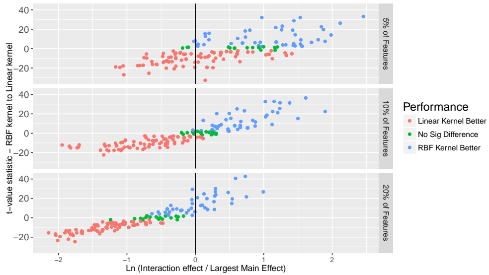
Figure 4.12.: Scatter plot showing the relationship between the median values of the log ratios of the interaction and respective largest main effect coefficients and the difference in performance of the RBF and linear kernels, assessed by pairwise t-tests; using the samples from both the I1M and OMNI chips. The colours represent if the difference in performance for the t-tests was significantly different at p < .05 , and which algorithm was performing better if the difference was significant.
