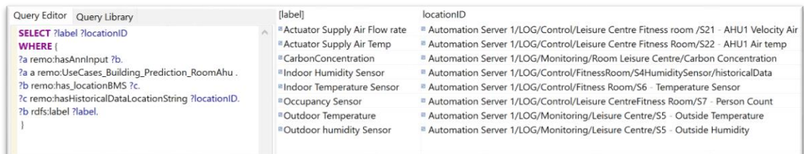
Figure 89. SPARQL query to retrieve ANN input for use case 1 and its results
