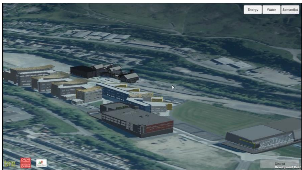
Figure 75. Screenshot of the visual interface showing 3D IFC model of buildings on the site
