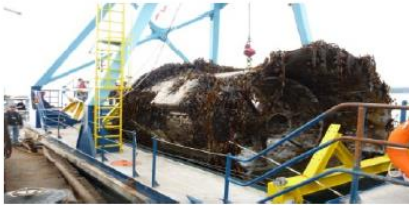
Figure 2.4: Condition of the Race Rock turbine after deployment (Elasha et al, 2013).
