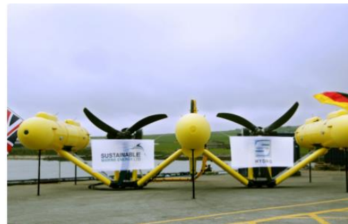
d) SME Plat-O incorporating Schottel Instream Turbines (SIT) (Sustainable Marine Energy Ltd, 2016)
