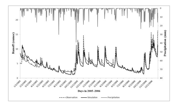
Figure 4-10 (c) Flow Calibration Sub - basin 9 (2005-2006)
