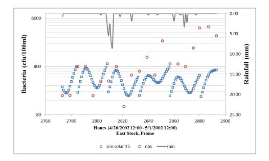
Figure 5-15 (c) Storm Event Validation with Solar Radiation Activate,
