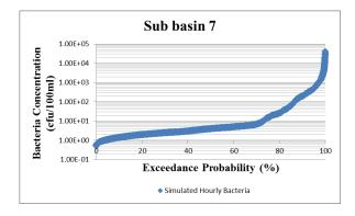
Figure 5-11 Simulated Bacteria (Hour) Duration Curve at Piddle Outlet
