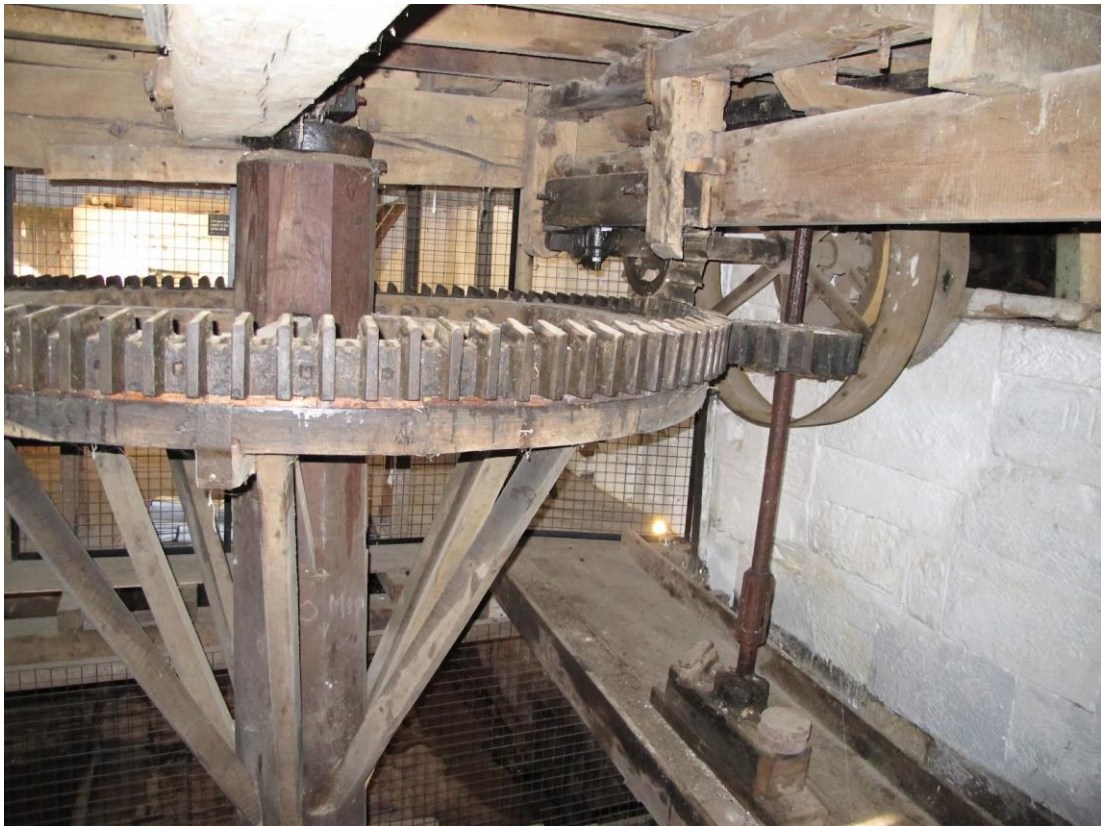
Figure 1.1 – Transmission of the Nether Alderley Mill dates from the 12th century as an example of the Vitruvius' watermills design
