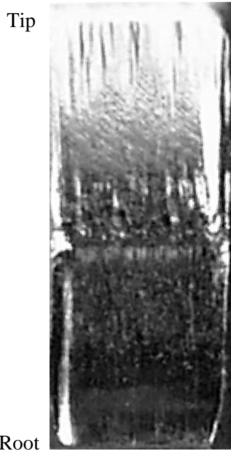
Figure 5.27 – Worn surface of the test gear tip to root (NASA/TM-2005-213956/ARL-TR-3126)
