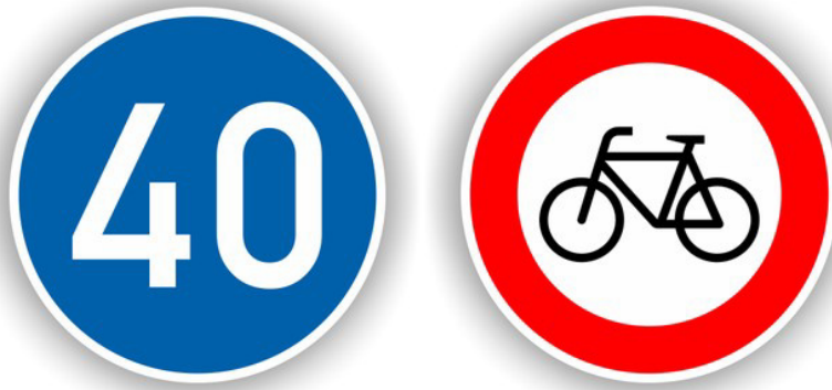
Figure 7. 18: Following the StVO sign 275 sets a minimum speed (in this case of 40km/h) and sign 254 prohibits cycling (Brewes GmbH, 2014)
