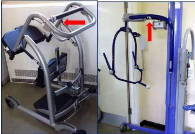
Figure 3. 14 Placement of tags on equipment (steady and hoist)
