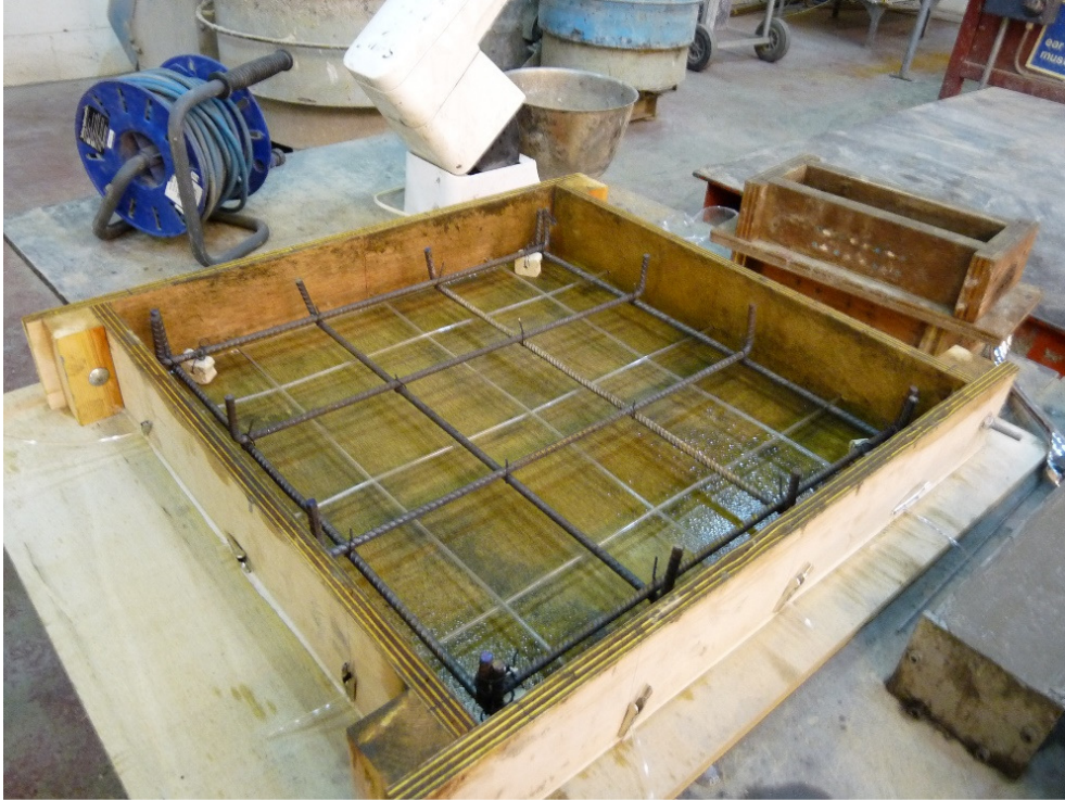
Figure 4: Vascular network channels before casting 600mm square 100mm deep slab
