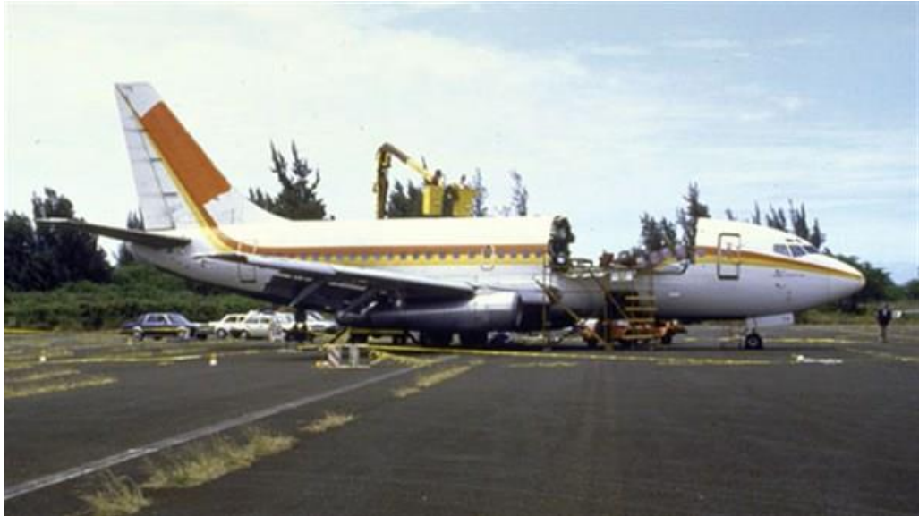
Figure 2: Boeing 737-200 Aloha Flight 243 showing significant structural failure.[3]
