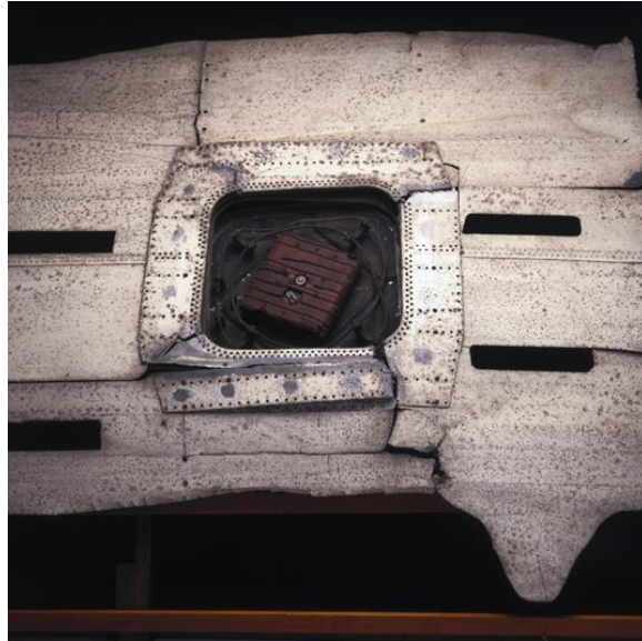
Figure 1: Wreckage of G-ALYP, one of the Comets that exploded mid-air, showing the fatigue cracks growing from the square windows. Currently on display in the London Science Museum.[2]
