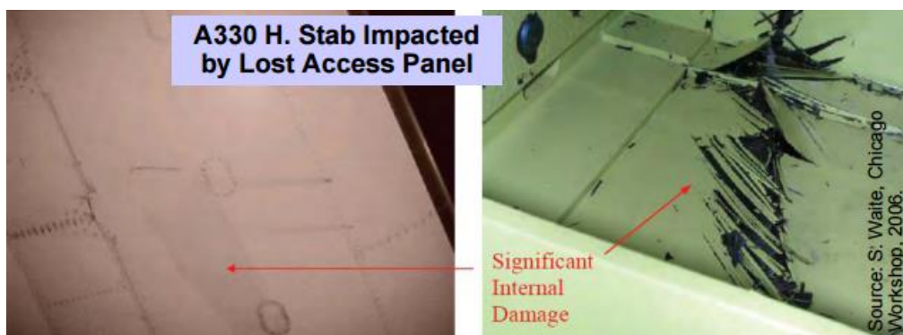
Figure 58. FOD caused by a lost access panel to an Airbus A330. Not that the extent of the damage is not apparent when viewed from the outside (reproduced from Kim [221]).
