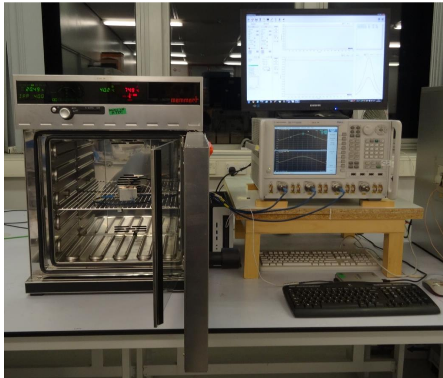
Figure 6.6: Photograph the bench-top experimental assembly. The sensor is put inside a computer-controlled oven and connected to an Agilent PNA-L N5232A network analyzer under LabVIEW program control.
