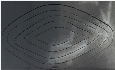
▲ Figure 15 Left: 2D pattern laser cut in concrete canvas. Right: Popped - up concrete canvas shell prototype
