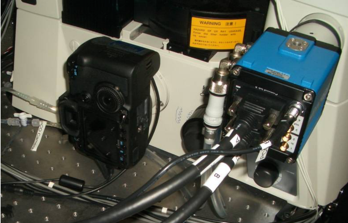
Fig. 2.1: Photograph of the left side of the Ti-U microscope. The 40D is attached to the left port of the microscope. The PCO is attached to the eye-piece side port.
