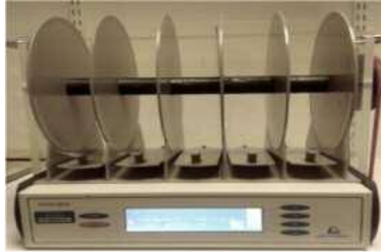
Figure 2.1. Photograph of the rotarod apparatus used in behavioural testing. The rotarod was manufactured by Ugo Basile S.R.I. 47600, VA, Italy.
