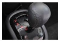
To start, depress the foot brake and release the parking brake. Far shift lever position "P" to "D" and go releasing the foot brake progressively, causing their movement was ahead.
