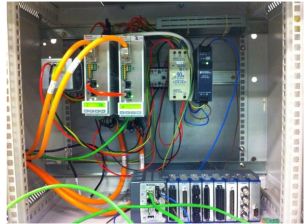
Fig. 14. The motor drives coupled via SERCOS III connection with an NI CompactRIO for making calculations and sending drive commands.
