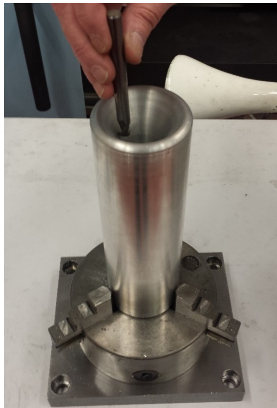
Figure 4.19: Photograph demonstrating the procedure of milling a curvature.
