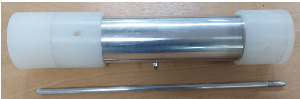
Figure 4.23: Prototype I with inner enclosure diameter of 30 mm and conductor diameter of 10 mm.
