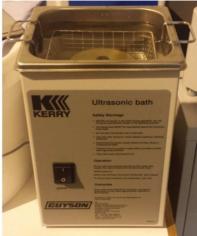
Figure 7.4: Ultrasonic bath for removing dirt on the surface of the electrode.
