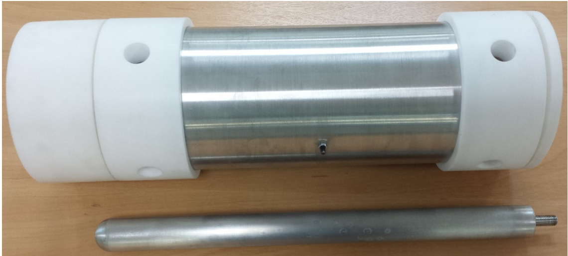
Figure 4.24: Prototype II with inner enclosure diameter of 90 mm and conductor diameter of 30 mm.
