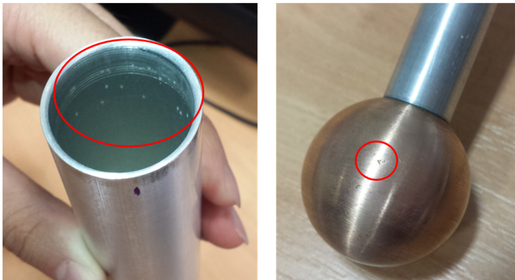
Figure 4.13: Markings on the enclosure wall and metal ball indicating occurrences of flashover around the edges of the enclosure.
