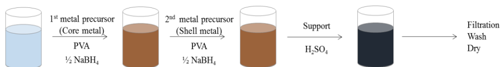
Figure 2.1: Sol-immobilisation preparation for Mono, Bi and Tri metallic catalysts
