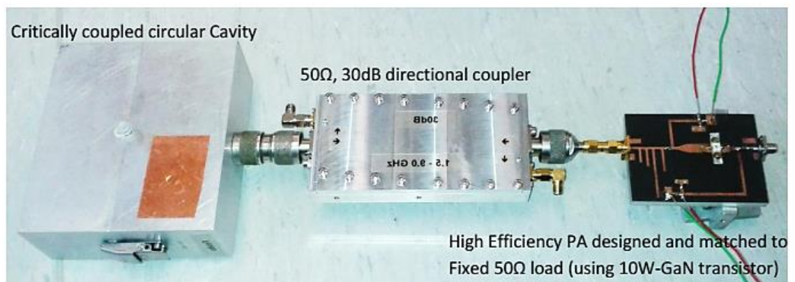
Figure 2: Conventional Solid-State Microwave Heating Apparatus with 10W-GaN PA and water loaded TM 010 mode circular cavity
