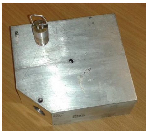
Figure 8.1: TM_{010} mode Cavity without coaxial connection (a hollow box)
