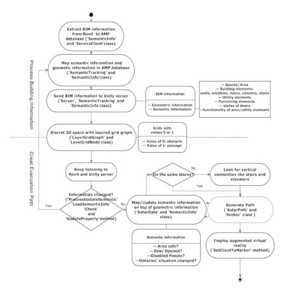
Figure 4.19 The workflow with associated classes and methods for the implementation of the path finding algorithm in the BIM-VE
