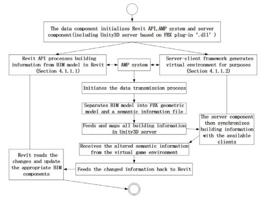
Figure 4.1 AMP system for two way information communication
