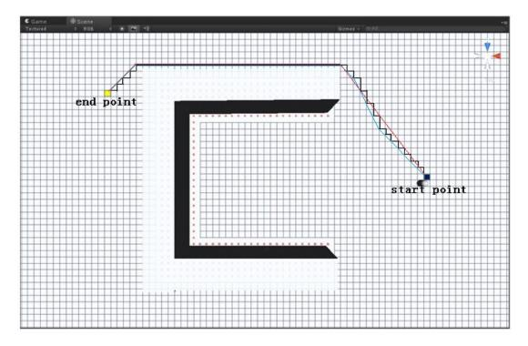
Figure 4.12 The shortest path generated by  $A^*$  algorithm with different h(x)
