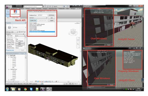
Figure 5.1 Autodesk Revit plugin to extract building information to the BIM-VE
