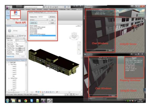
Figure 5.16 Automatic data transmitting between Revit, the Unity3D server and the Unity3D clients
