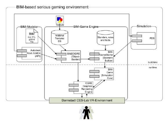
Figure 2.8 BIM-based serious gaming environment (Rüppel and Schatz 2011b) *Torgue:* Three main steps were involved for developing BIM-Game workflow based on Torque Game Engine (TGE) (Shiratuddin 2011). Step 1 was modeling of the
