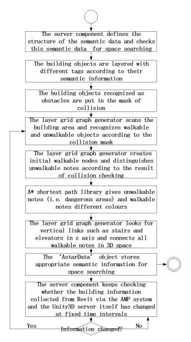
Figure 4.20 Workflow to create preliminary coloured 3D discretised space for shortest evacuation path
