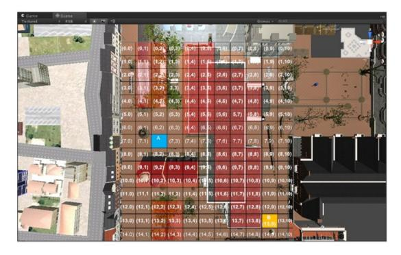
Figure 4.17 Define the world within the grid coordinate (obstacle tiles in red colour area)
