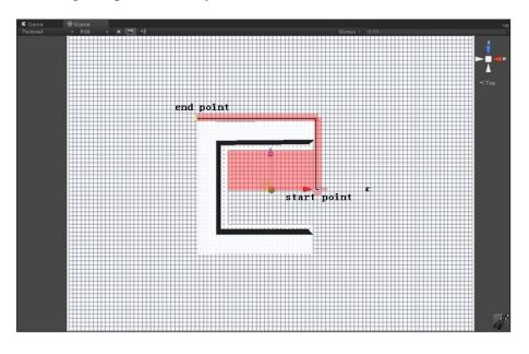
Figure 4.11 The shortest path from start point to end point based on A\* space searching algorithms
