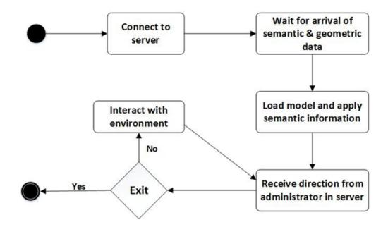
Figure 3.6 Client end work flow
