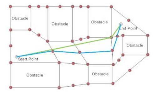
Figure 4.15 Hybrid shortest path generation based on navmesh graph
