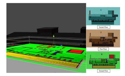
Figure 4.21 Layered grid of nodes and marked obstacles in the multi-floor building (green, brown and blue grid of nodes for walkable area, red nodes for obstacles, yellow grid of nodes for closed spaces)
