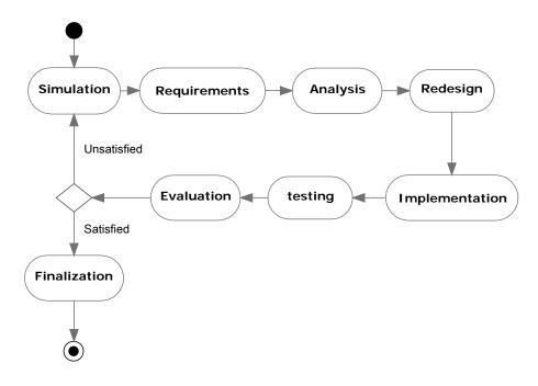
Figure 4.40 The interactive steps to refine building designs by the evacuation behaviour simulation
