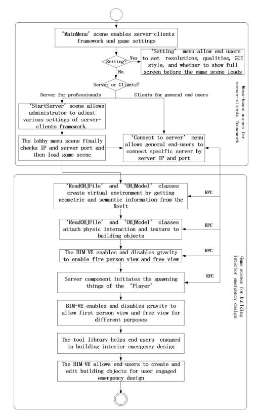
Figure 4.27 The workflow to get end users engaged in emergency design 136
