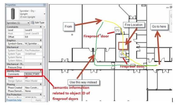
Figure 5.20 The scenario of the fire alarm works with semantic information to automatically change the fire evacuation path ((1) and (2) are fireproof doors which IDs are 381844 and 373405 and referenced to the fire alarm/sprinkler; yellow route is original evacuation path and the green route is the alternative path when fire alarm is activated)
