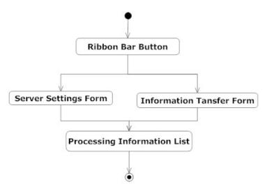
Figure 4.3 The appear order of forms contained in the Revit plugin
