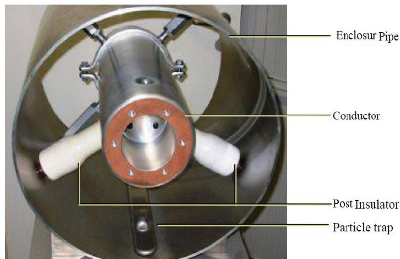
Figure 2-1: Overview of Single Phase GIL Pipeline [20]
