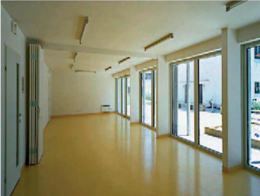
Picture 2: Inside a passive house in Germany. The building is well insulated and optimized for natural light. The only radiator in this spacious hall is never used unless the outdoor temperature falls very low.
