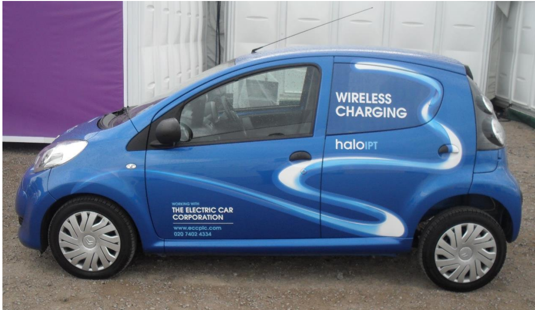
Figure 101 - Citroen C1 ev'ie fitted with Halo IPT Inductive Power Transfer
