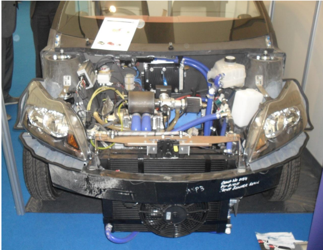
Figure 95 - Front end, with body panels removed, of Axon Hatchback. Note extensive use of carbon fibre, and novel chassis technology.
