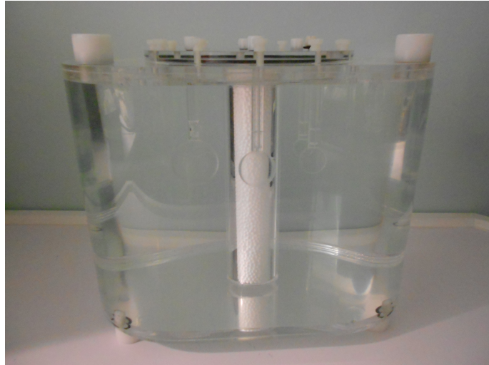
Figure 4. Picture of the filled NEMA IEC body phantom with central lung insert.
