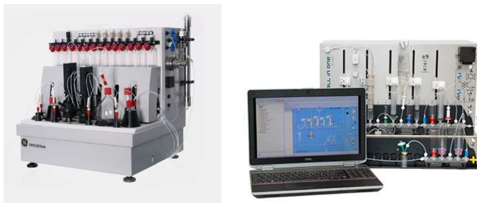
Figure 13: GE TracerLab FX N Pro module system (left) and the Trasis All-in-One system (right).
