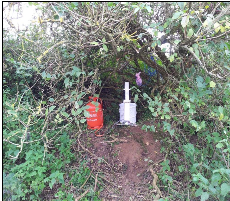
Figure 8.13: A CO 2 Generator placed at one of the test sites having ideal conditions for mosquito breeding
