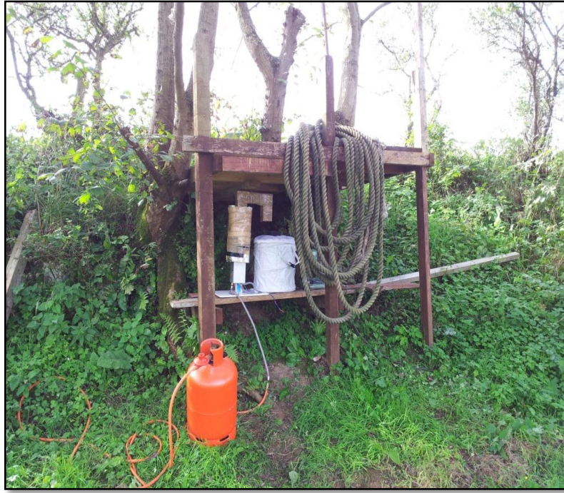
Figure 8.12: A CO 2 Generator connected to a 13 kg propane bottle, placed at a test site near Swansea
