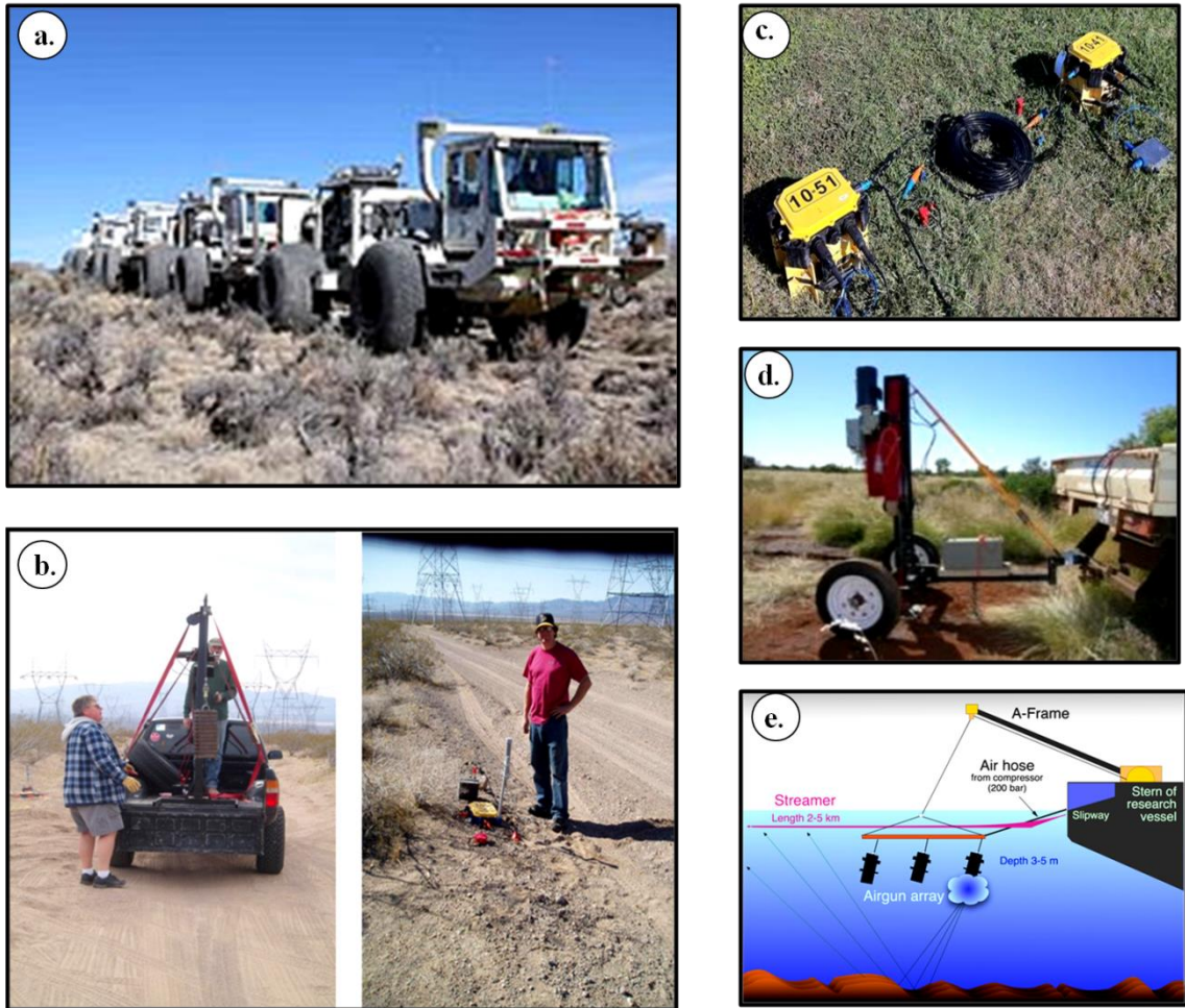
Figure 3.2: Examples of seismic acquisition sources (a.) Vibroseis in a set ( http://www.cflhd.gov ) (b.) Weight dropping and sledge hammer ( http://mettechnology.com ) (c.) geophones ( http://iseis.com ) (d.) weight dropping ( http://geophysics.curtin.edu.au ) (e.) Air gun used for marine survey ( http://upload.wikimedia.org/wikipedia/commons/1/1d/Airgun-array_hg.png ).
