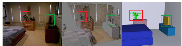
Figure 16: Higher \lambda_c helps recover objects with lower classification confidence (e.g. the TV set), but causes misidentification of point clouds that should be rejected by the classifiers (e.g. the plants).
