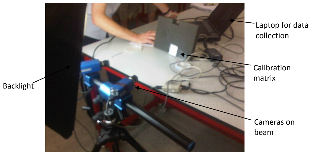
Figure 6.11 Calibration and system set up for digital image correlation.
