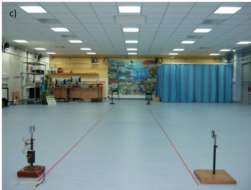
Figure 2.13 a) A typical motion capture camera, with a ring of infra-red LED's around an infra-red camera. b) A patient fitted with retro-reflective markers (consent has been obtained to use these images). c) The motion analysis laboratory used in one of the studies (ORLAU, Oswestry). The patient walks along the walkway whilst the 12 cameras simultaneously record motion of the reflective markers.
