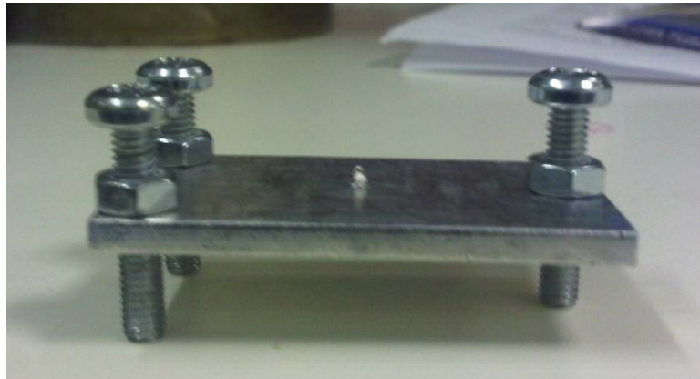
Figure 6.4. One of the two identical tilt tables used in this study, designed and made by Professor Evans. Both had an aluminium plate with a small spike in the centre (a Kirschner-wire tip) which had been driven through the plate and protruded by 1.5mm, which was used to stabilise the subchondral cancellous bone to prevent horizontal slippage of the core during testing. The angle of the plate could be adjusted in any plane by adjusting the length of the tripod screws individually.
