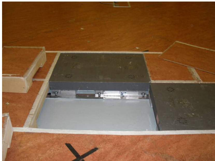
Figure 2.14. Two force plates built into the floor. The surrounding removable boxes and vinyl covering are also pictured, so that when in place the surface of the force plate is continuous with the floor.
