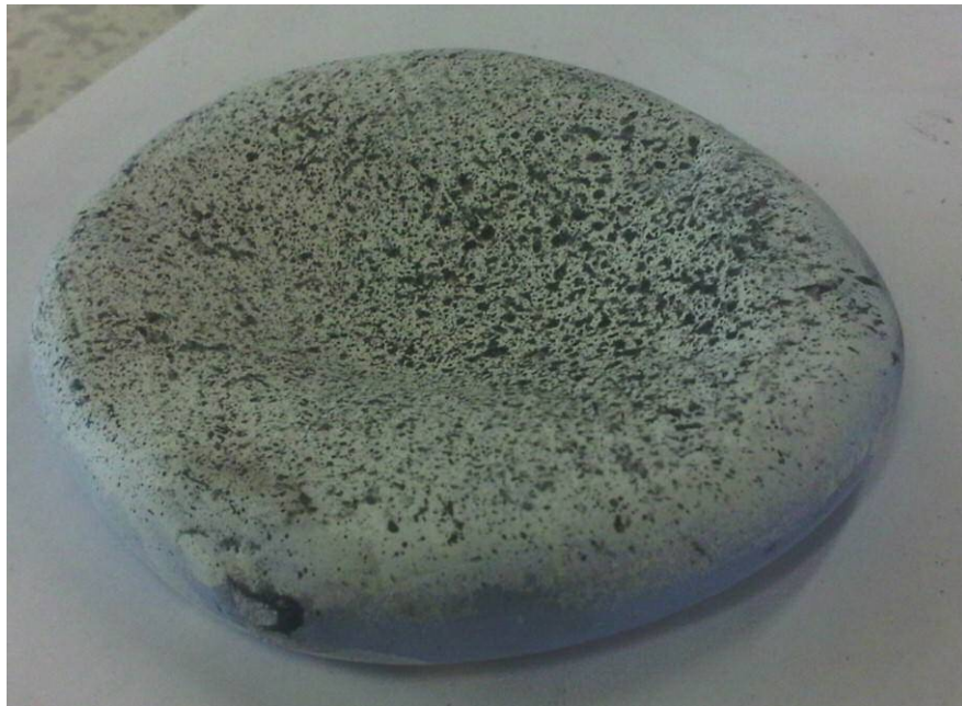
Figure 6.10 Example of mould covered with speckle pattern
