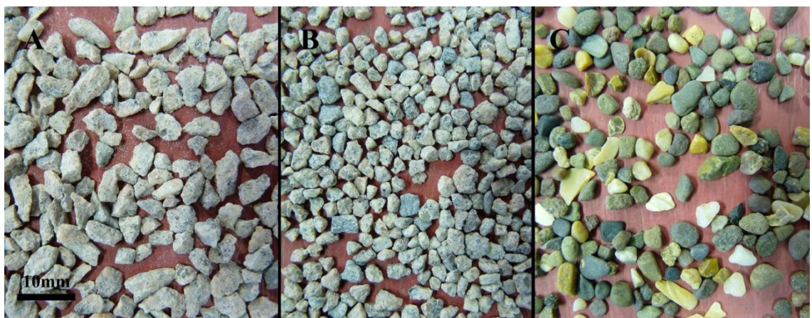
Figure 3.5.8 Images of 4-2 mm sand fractions, A: G-FEED, B: G-A, C: NS.
