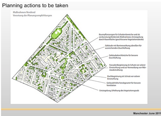
Frankfurt, point-specific design recommendations based upon high-resolution climate analysis. Image, Professor Lutz Katzschner, Kassel University
