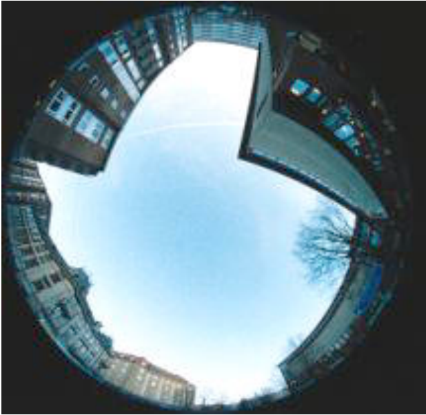
Figure 18: Fish eye image used for measuring sky view factor (SVF), http://www.gvc2.gu.se/ngeo/urban/Activities/svf.htm (2009).
