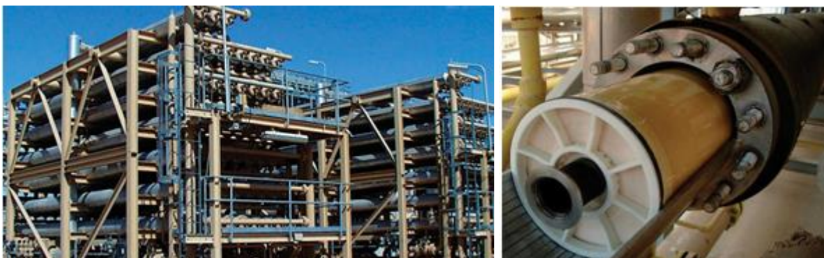
Fig 2.2c. UOP Separex™ membrane system in Egypt. Two of five racks shown (left), A single module (right).
