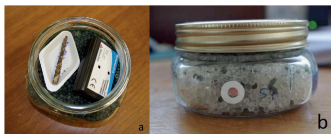
Figure 1: Set up of oxygen measurement system; a) the object and RH/temperature logger sit on a bed of conditioned silica gel to control humidity; b) the sensor spot (pink) adhered to the inside of the jar using transparent silicon adhesive allows measurement through the glass.
