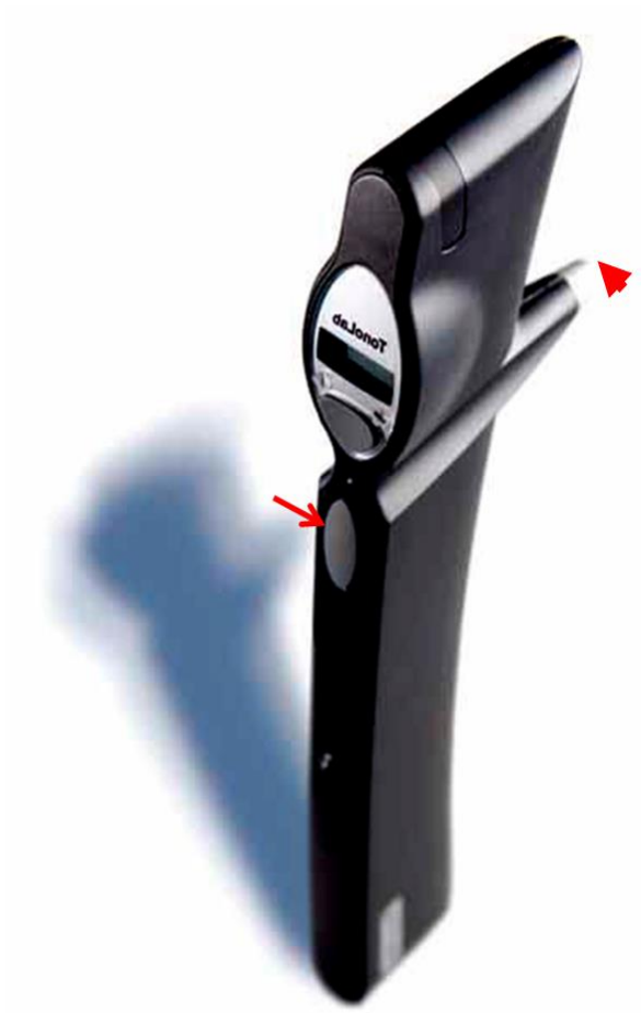
Figure 2.2 The Tonolab® tonometer. The trigger (arrow) is pressed to activate probe (arrowhead) which contacts the animal's cornea to take a measurement of the intraocular pressure. (Image from TioLat, Finland). The placement of the activation button on the handle allows for single-handed operation, leaving one hand available for gently restraining the animal which is being measured. The small contact surface of the probe (1mm in diameter) allows for measurements to be taken solely from the centre of the cornea, preventing any confounding effects which may be produced by the probe striking microspheres in the iridocorneal angle.
