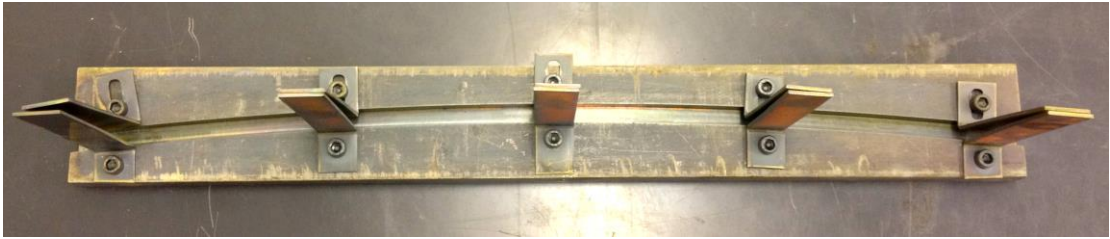
Figure 6- 3: The design jig for applying different curvature, a set of 10 samples were clamped in a jig and annealed at 810°C for 2hrs.
