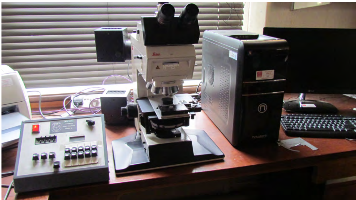
3.2. Point counting apparatus: Leica DMR microscope, Swift automatic pointer with modified mechanical stage.
