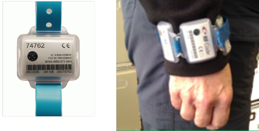
Figure 5.1: Active IR-enabled RFID Tags
