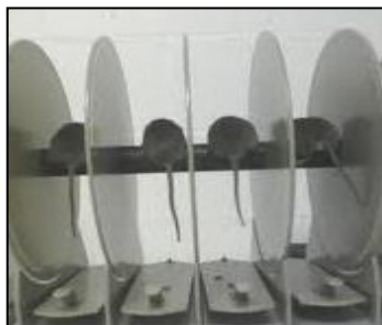
Figure 2.5 Mouse Rotarod apparatus. 5 mice were tested on the apparatus simultaneously. When the animal's fall onto the panels at the bottom, the automated counter stops and re-sets to 0.
