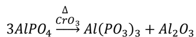
Equation 3.11 The formation of aluminium metaphosphate from aluminium orthophosphate during heating in the presence of chromium trioxide
