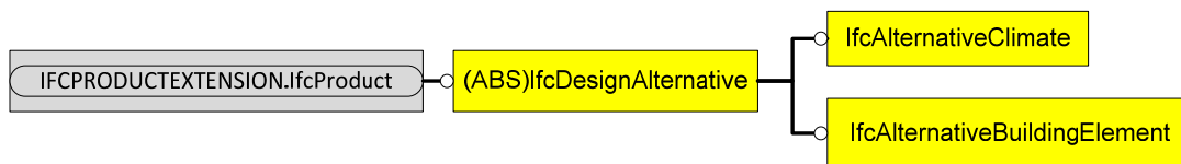
Figure 5.7 An EXPRESS-G diagram of the proposed ' IfcDesignAlternative ' entity.
