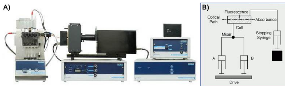
Figure 2.7 Example of a stopped flow instrument (A) and the principle of its mechanism (B).
