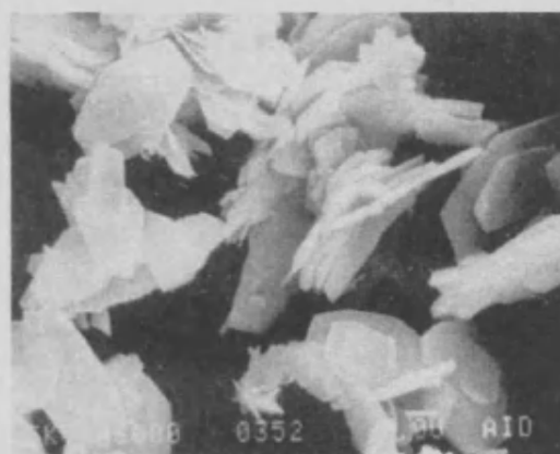
Fig. 1.20: SEM image of (VO)_2P_2O_7 after dehydration of the precursor in Fig 1.19 [73]
