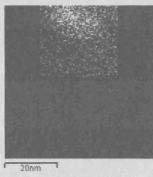
Fig. 4.27: STEM of Au/Pd 95/5 catalyst Cl map
