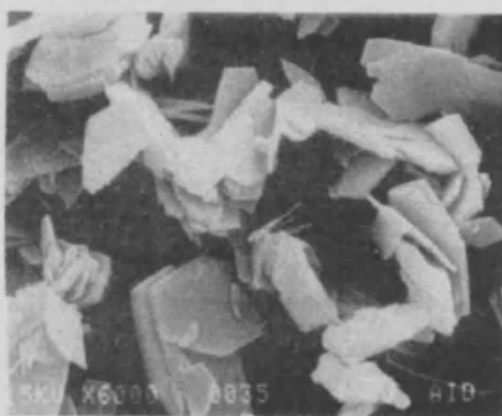
Fig. 1.19: SEM image of VOHPO_4 \cdot 0.5H_2O prepared in butanol solvent [73]
