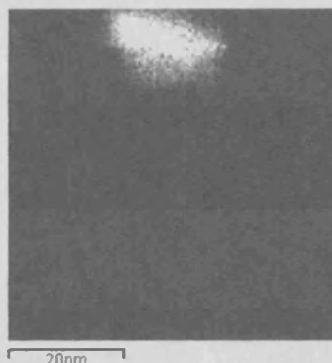
Fig. 4.25: STEM of Au/Pd 95/5 catalyst, Au map
