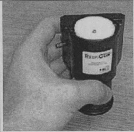
Figure 4.7h : Lift Body Unit to Cover Filter Stages.
