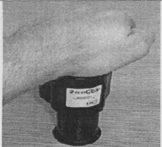
Figure 4.7d : Press Down to Remove Filter Stages.
