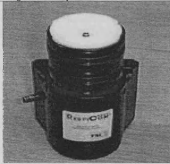
Figure 4.7g : Place Body Unit Over Removal Cylinder. Place Stacked Filter Stages into Body Unit.
