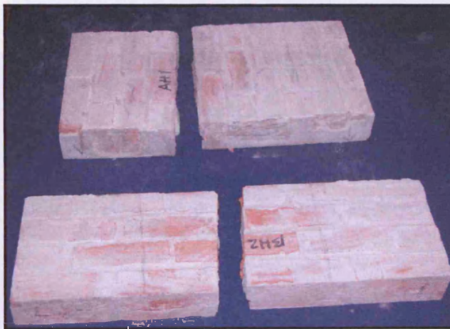
Plate 5.5- Failure in half scale flexural strength specimens.
