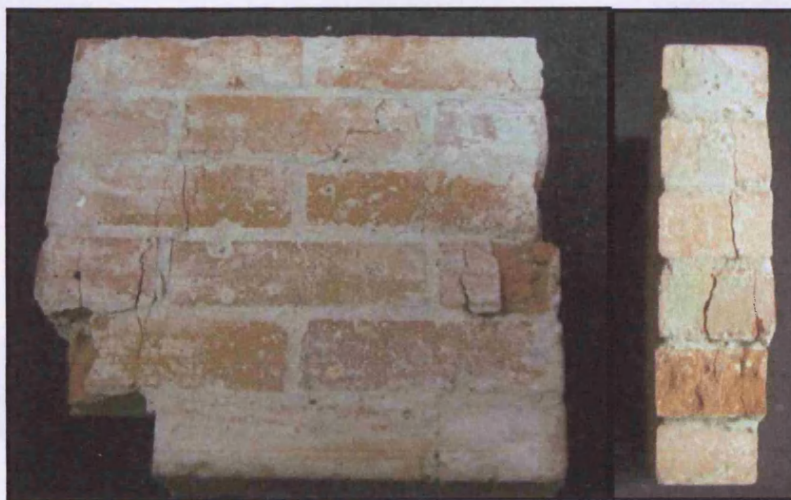
Plate 5.3- Cracking patterns in sixth scale wallettes.
