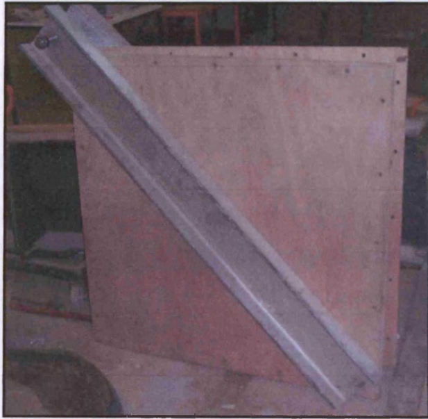
Plate 4.11- Wooden panel used for carrying the prototype diagonal tensile strength test specimens.
