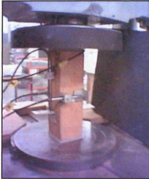
Plate 3.2- Set up of brick modulus of elasticity test.
