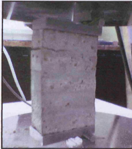
Plate 7.4- Bond failure in top bed joint of model specimen at e/d of 0.39.
