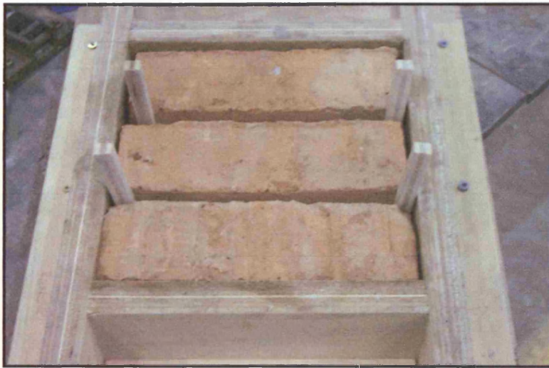
Plate 3.1(a)- Triplet masonry specimen in preparation.
